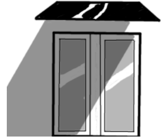
Figure 1: Schematic representation of a window with an overhang. In this paper the overhang used are active BiPV components
