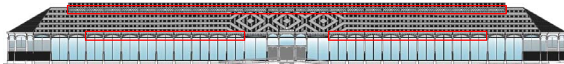
Figure 4: South-west front view of the building where openings locations are highlighted in red.
