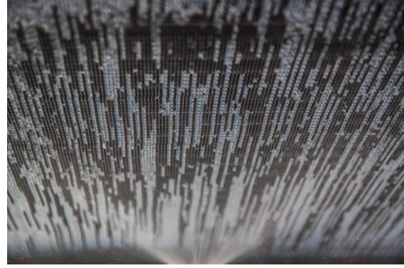
Fig. 2 – Picture of the 1st row (bottom part) of the coil while sprinklers are active
