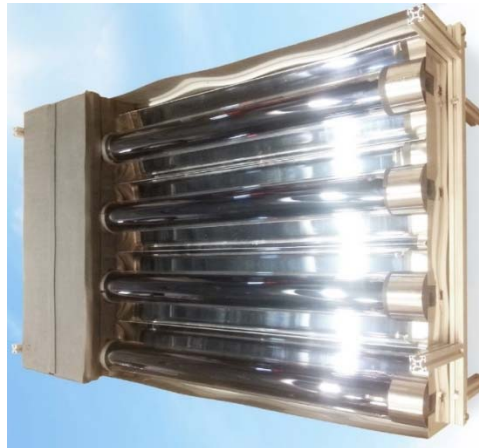
Figure 1: View of the prototype of the sorption collector [source: ClimateWell].
